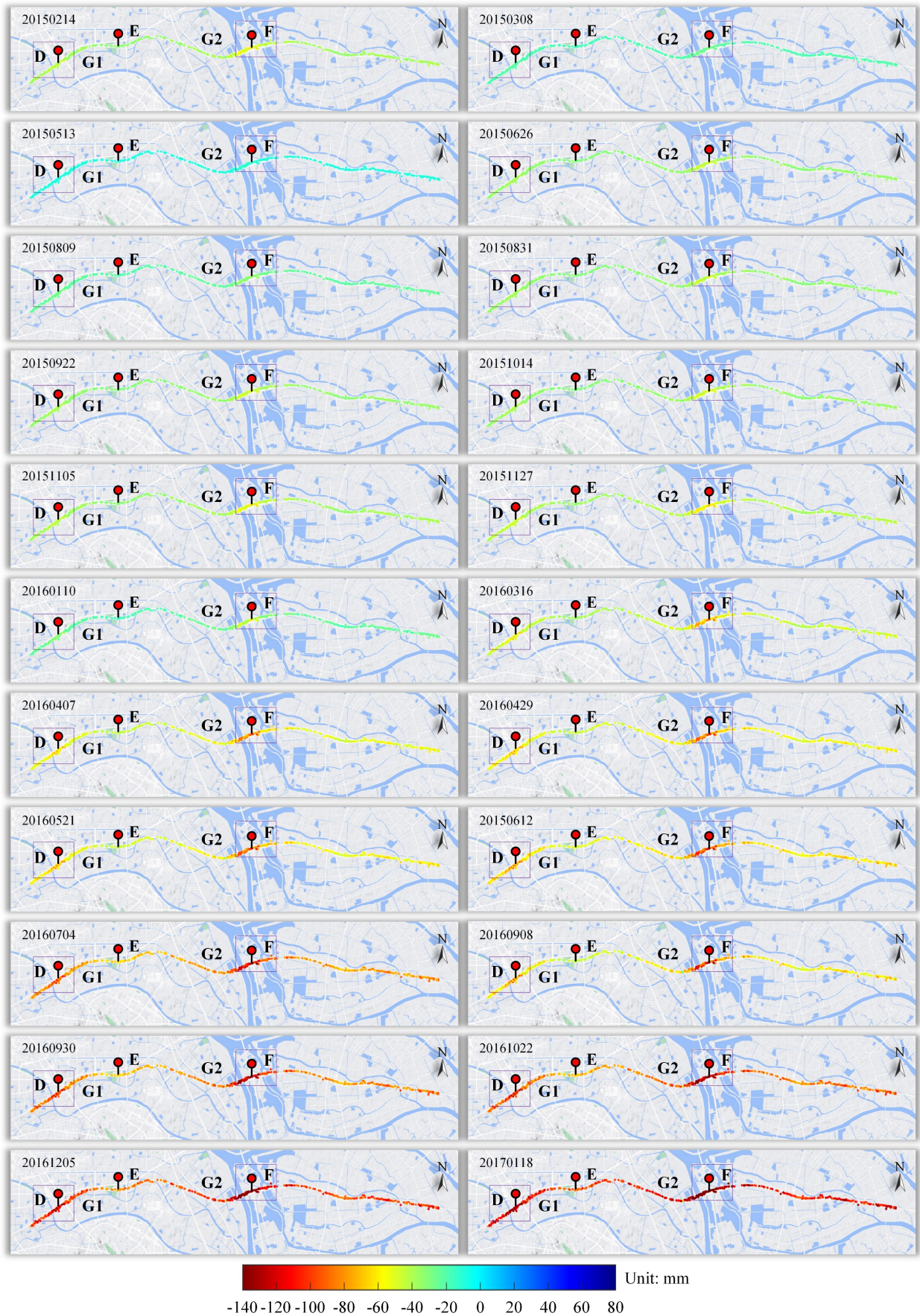
Fig. 11. Generated deformation sequences of the GH (with reference to 01/01/2015; D-F represent the locations of feature points).
